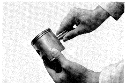
Fig. 6-6-3 Inspecting piston pin holes
